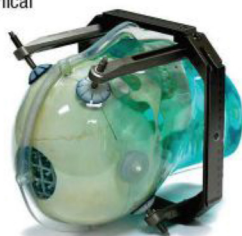
Inter-Cranial Grid Phantom 335 Physical Control Points
